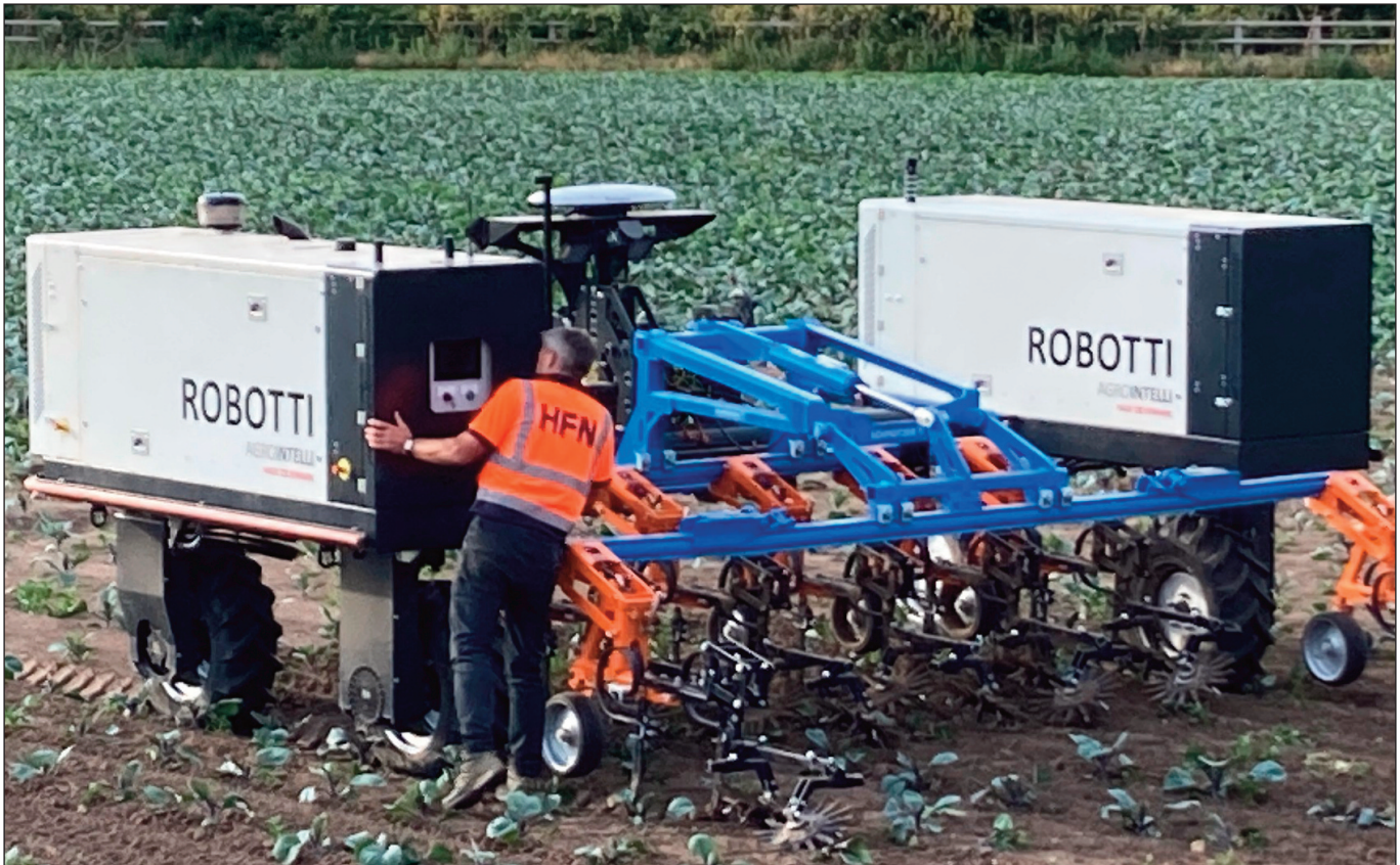
Andrew Williams demonstrating one of the Robotti automated machines that can weed day and night unmanned, controlled by GPS, lasers and a clever computer program
